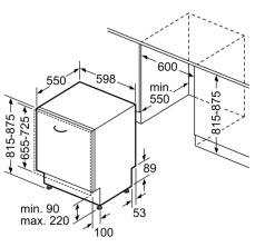
measurements in mm
