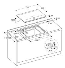
A:  $6.5^{\circ,0.5}$  B: Please check the installation manual if the worktop depth is less than 600 mm.
