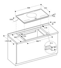
A: Please check the installation manual if the worktop depth is less than 600 mm.
