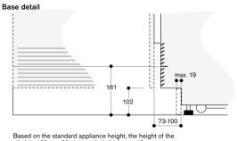
Based on the standard appliance height, the height of the plinth is 102 mm. Maximum plinth thickness 19 mm.
