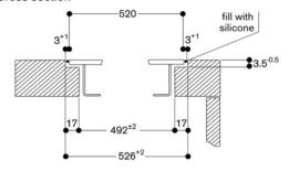
When installing with appliance cover or spacer batten, pay attention to the deeper cut-out and the front and rear groove width.
