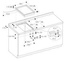
A: When installing with appliance cover, take the deeper cut-out into consideration (observe separate planning notes) B: 133 mm in the area of the cable clamp (left, on the rear side) C:  $3.5^{\circ5}$
