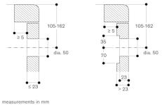
Installation with appliance cover, surface mounting
