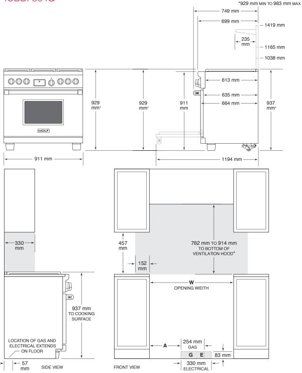
\*Without ventilation hood, 914 mm minimum clearance countertop to combustible materials, 118 mm for charbroiler. NOTE: Shaded area above countertop indicates minimum clearance to combustible surfaces, combustible materials cannot be located within this area.
