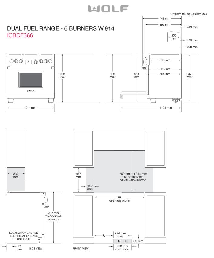
\*Without ventilation hood, 914 mm minimum clearance countertop to combustible materials, 118 mm for charbroiler. NOTE: Shaded area above countertop indicates minimum clearance to combustible surfaces,
