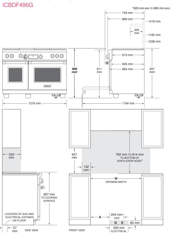
\*Without ventilation hood, 914 mm minimum clearance countertop to combustible materials, 118 mm for charbroiler.
