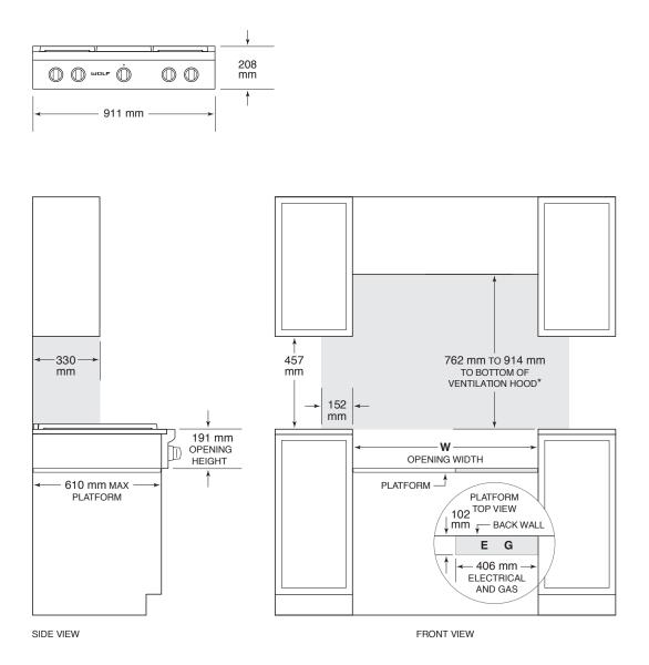
\*Without ventilation hood, 914 mm minimum clearance countertop to combustible materials, 118 mm for charbroiler.
