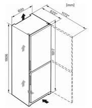
KF28033D, KF28032, KFN28032, KFN28032D edt/cs, KD28032, (installation drawings) (\*footnote)
