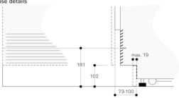
In relation to the standard height of the appliance, the height of the toe kick plate is 102 mm. Maximum thickness of the toe kick plate is 19 mm
