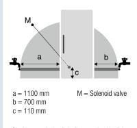
Plumbing must be installed adjacent to the side of the appliance which contains the IceMaker. Water pressure must be between 0.15 MPa and 0.6 MPa (1.5 bar - 6 bar)
