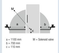
Plumbing must be installed adjacent to the side of the appliance which contains the IceMaker. Water pressure must be between 0.15 MPa and 0.6 MPa (1.5 bar - 6 bar)
