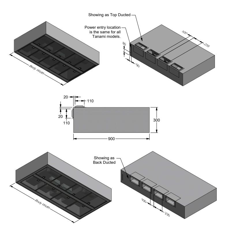
Tanami comes top ducted and can be converted to back ducting on site by the installer.
