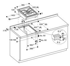
A: When installing with appliance cover consider the deeper cut-out (observe separate planning notes) B:  $3.5^{\circ 5}$
