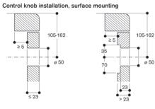
measurements in mm
