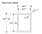
A: When installing with appliance cover consider the deeper cut-out (observe separate planning notes)
