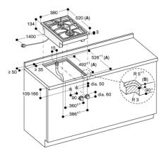
A: When installing with appliance cover consider the deeper cut-out (observe separate planning notes) B:  $3.5^{\pm a}$
