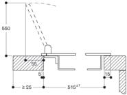
Measurements in mm
