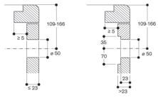
measurements in mm
