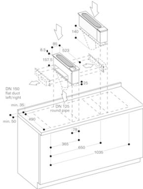
Flat duct pipe connection piece, left/right
