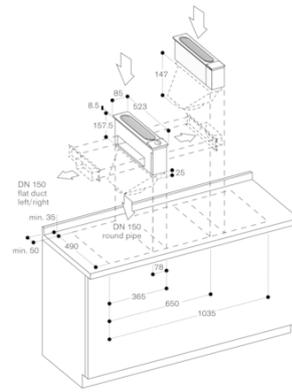
Flat duct pipe connection piece, left/right
