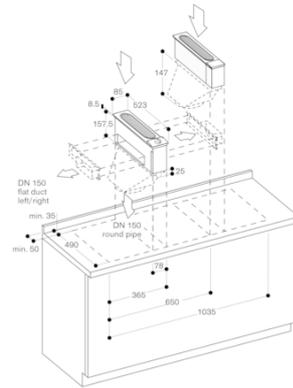
Flat duct pipe connection piece, left/right
