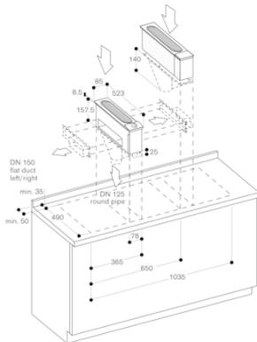
Flat duct pipe connection piece, left/right
